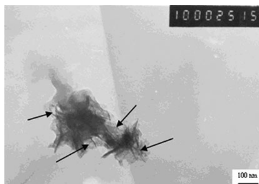
Fig. 5 TEM photos of PVA/OMMT2 milled for 60 pan-milling cycles
