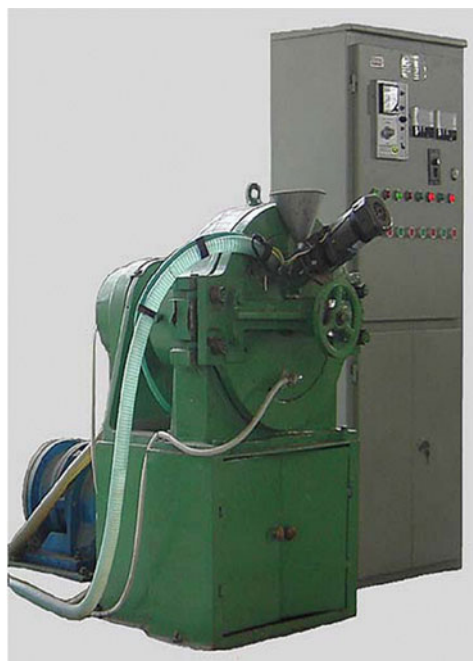
Fig. 1 Digital photograph of the pan-mill type mechanochemical reactor
